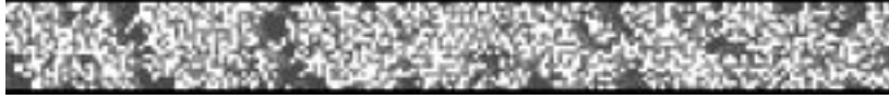
Fig. 3.6. Density for a square lattice with periodic boundary conditions and global density \rho = 4.4 \text{ P/m}^2 . The occupied cells are indicated by dark, the empty by white dots. Jam waves moving opposite to the walking direction, which is from left to right, can be observed.
