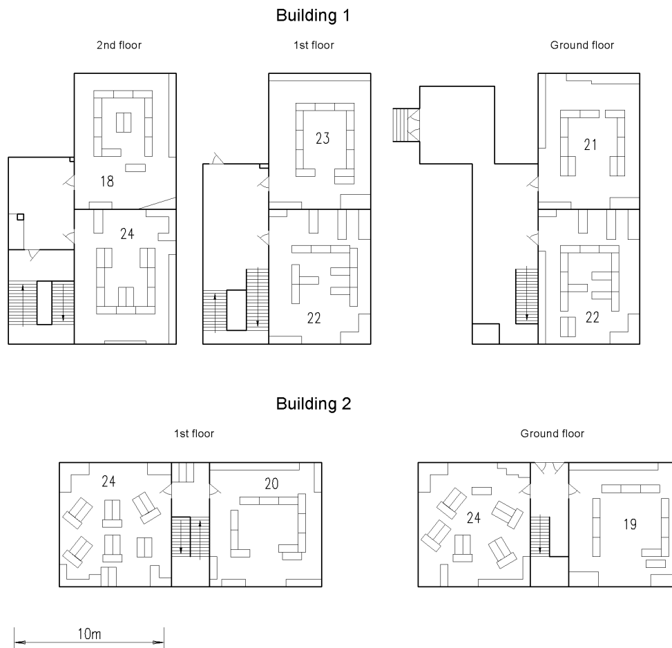
Fig. 4.8. Layout of the school building. It is separated into two independent parts (building 1 and 2), building 1 having three, building 2 two floors. The numbers show the initial number of persons in the rooms according to the class sizes. The pupils gather on the playground just in front of each building.
